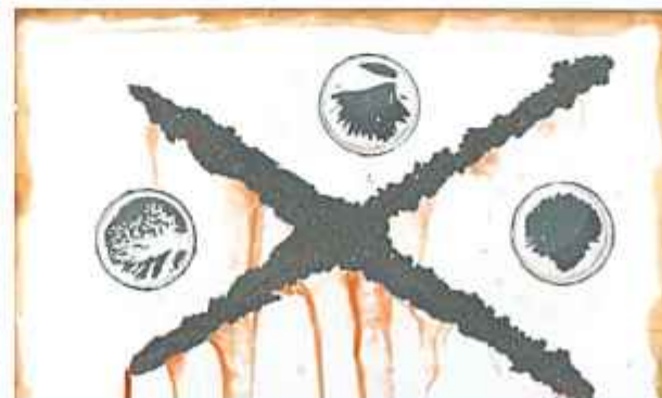
After 1500 hr salt spray test
