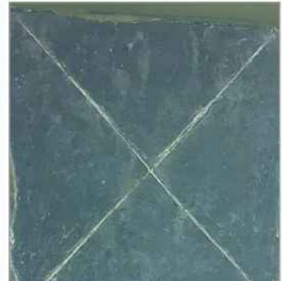
Cool Galvanizing Coating after 1500hr Salt Spray Test
