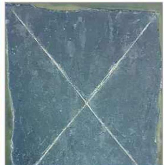
Cool Galvanizing Coating after 2500hr Salt Spray Test
