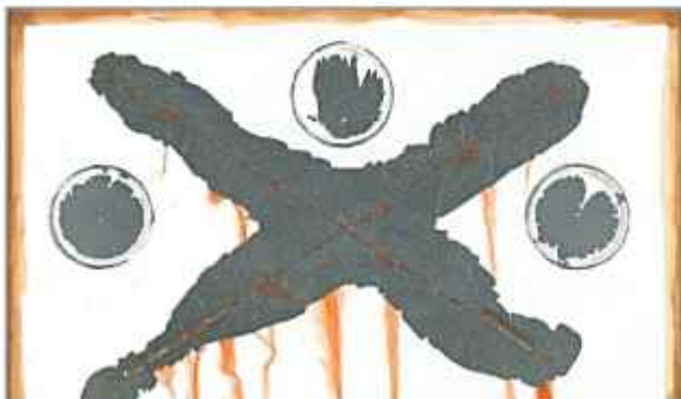
After 2500 hr salt spray test
